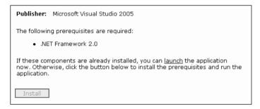
**Figure 7-19.** The publish.htm script detects that the .NET Framework 2.0 is not installed on the target machine.
