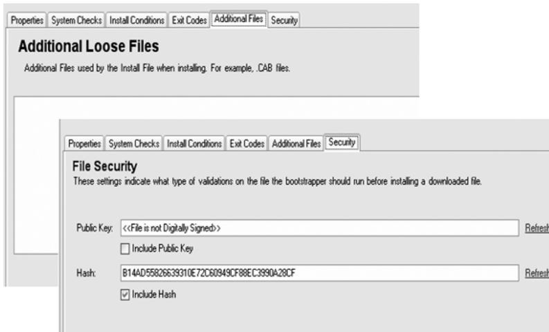
**Figure 9-9.** *Configuring additional files and security with the BMG*
